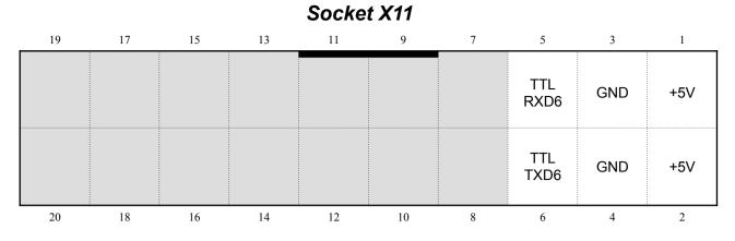
This socket is used for external devices (bill acceptors) with interface with direct TTL logic: 0 - 0V, 1 - +5V. Some manufacturers of bill acceptors (CashCode) uses name "Opto-isolated" to call it.
